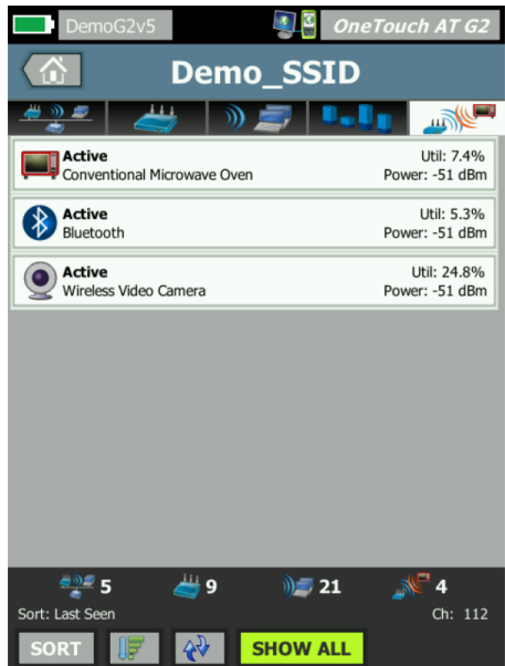
Figure 15. Unique Interferer analysis classifies sources of non-802.11
