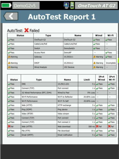
Figure 22. Detailed breakdown of network service performance
