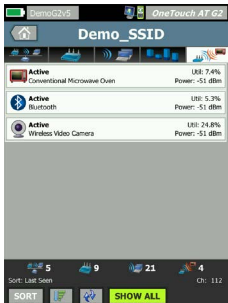
Figure 15. Unique Interferer analysis classifies sources of non-802.11
