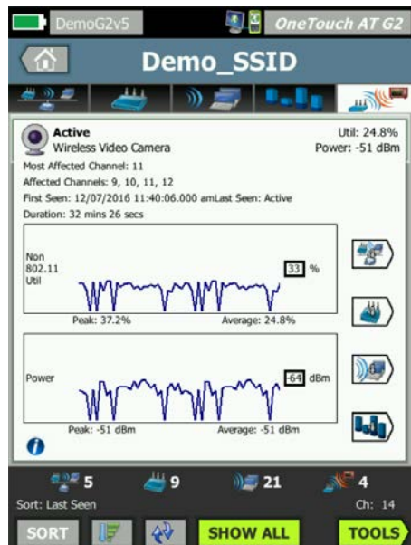
Figure 16. Detailed information about a specific interference source
